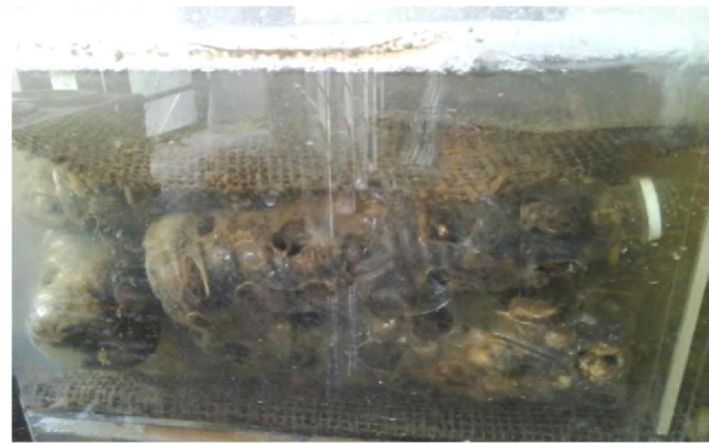
Fig. 2: The media fills along with mesh support inside the reactor.
