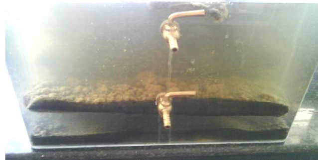
Fig. 3: The biomass growth inside the reactor.
