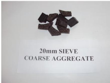
Fig. 1: Waste tyre rubber replaced for coarse aggregate.
