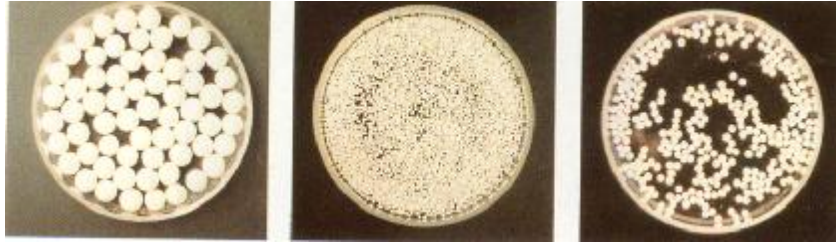
Fig. 10: Ceramic beads covered with titanium dioxide to kill bacteria
