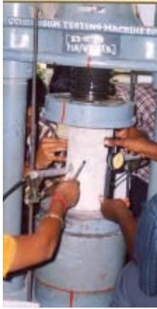
Fig. 6: Strain measurement using DEMEC.
