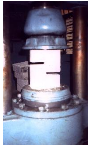
Fig. 2: Test setup for shear strength.
