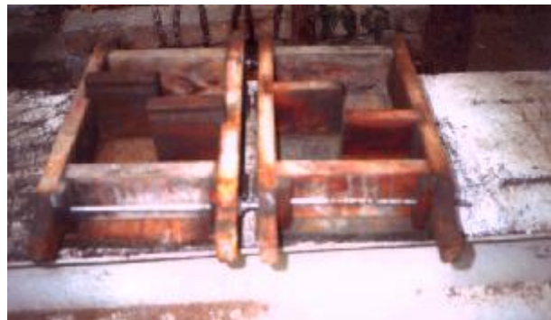
Fig. 1(b): Shear moulds.
