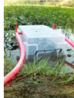
Fig 1. Collection of methane using gas chamber with two cocks connected to gas bladder.
