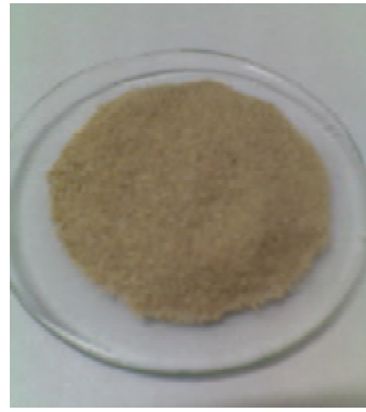
Fig. 2: Prepared rice husk as adsorbent (300-150µm)
