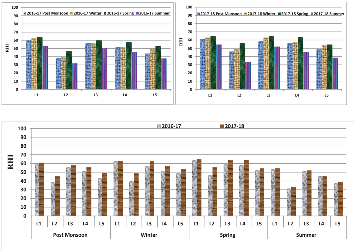
Fig. 3: Variation of River Health Index (RHI) for River Ganga at different locations near Varanasi during 2016-2017 and 2017-2018.
