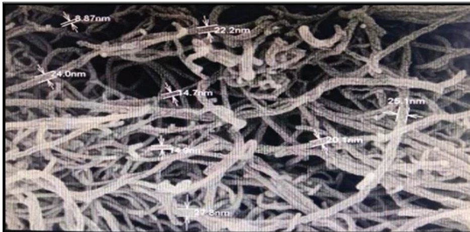
Fig. 1: TEM image of carbon nanotubes.
