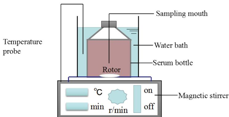
Fig. 2: Schematic diagram of the batching test.
