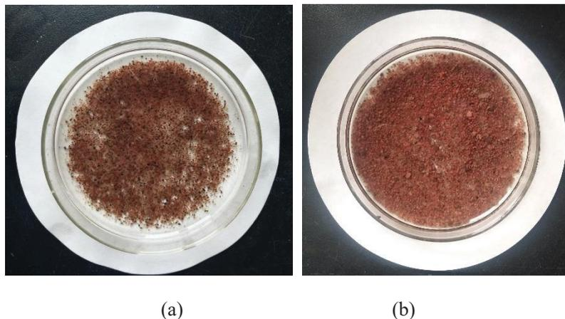
Fig. 5: The variation of anammox granular sludge in (a) 0 d and (b) 159 d.
