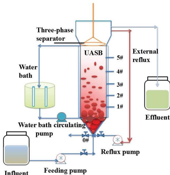
Fig. 1: Schematic diagram of the anammox granular sludge-based UASB reactor.
